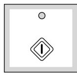
This button has three functions: Start - Pause - Draining of water/Spin
